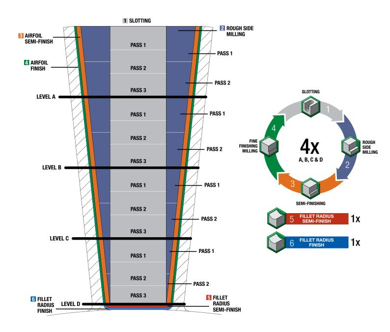
The WIDIA-Hanita™ end mills IBR machining tools are specifically designed to match a multi-level machining process for the airfoils, followed by the fillet feature, which works for roughing and finishing operations. In this machining strategy, the opening is machined on 4 levels, simultaneously creating the opening and finishing the sides of the airfoil at the desired surface finish requirements.
